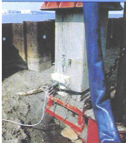
Fig. 4. Dynamic load capacity testing equipment.
