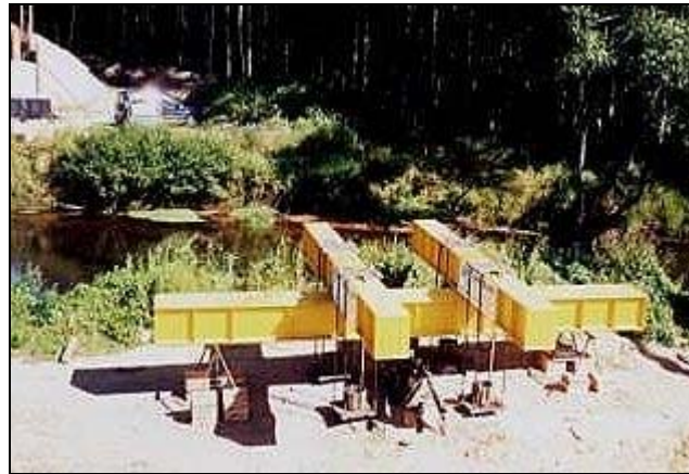
Fig. 1. Static load testing stand.
