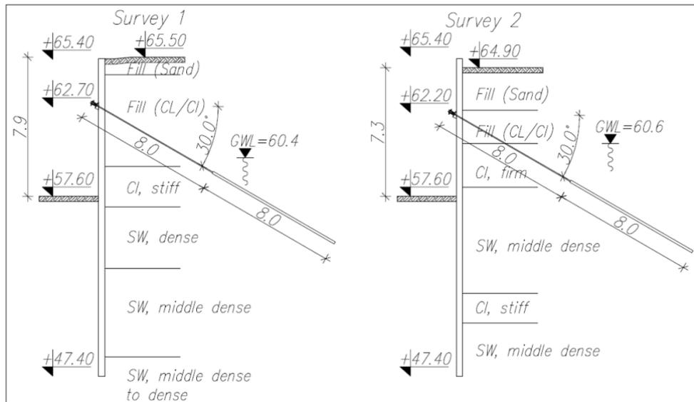
**Fig. 3. Sheet pile wall cross section at survey locations**
