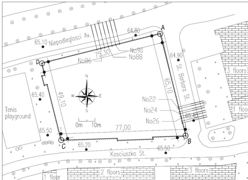
**Fig. 1. Excavation with the surroundings and survey layout**
