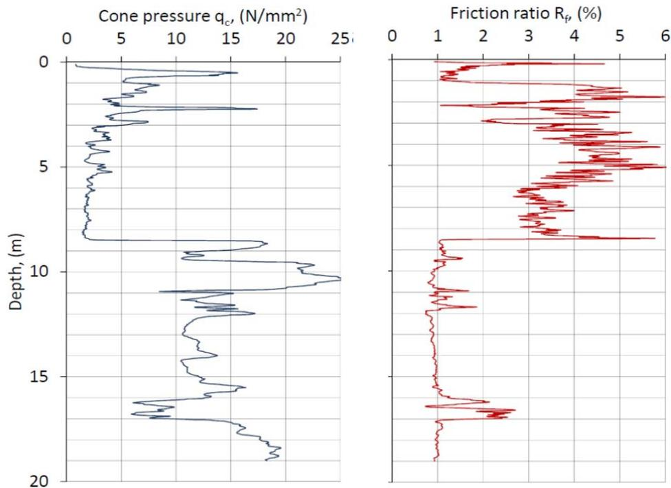
**Fig. 2. Cone pressure and friction ratio from CPT10**
